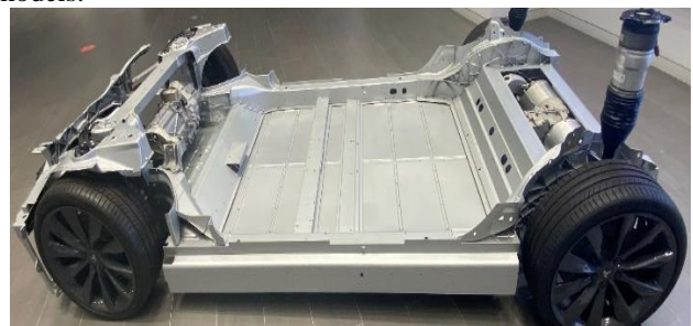
Fig. 1. Tesla Model-S Chassis with Batteries and Motors [2]
