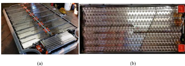
Fig. 3. (a) Represents the Tesla Models-S Assembled Battery Pack and (b) Individual Pack [31]
